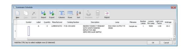
A default **Symbol** will be created for the new item based on the luminous opening dimensions included in the *photometric file* and not the physical dimensions of the entire *luminaire*. The *symbol* dimensions can be modified if necessary; see <u>The Symbol Editor</u>.
